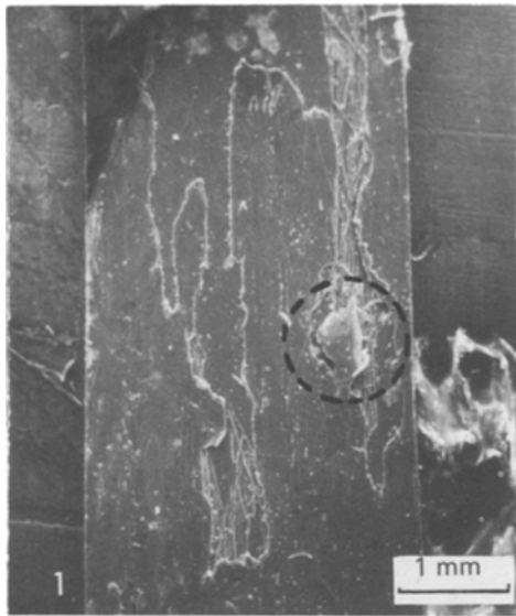
Figure 8 Tearing and splitting of metallized polycarbonate film at the surface of a lamella produced by the fracture of a sample. (1) General view of the lamella. (2) Detail of the circle in (1). Subadjacent fibres can be seen.
